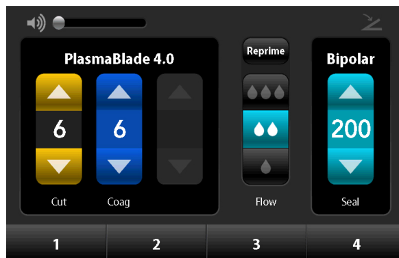
Figure 3-8. Front Panel Displaying the Screen with PlasmaBlade™ and Bipolar Handpieces Connected and activated.
